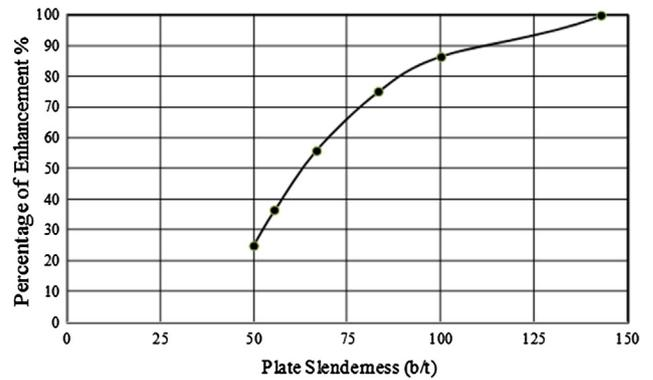
**Fig. 20a.** Variation of strength enhancement percentage with plate slenderness ratio for fully wrapped square hollow section (100 × 100 mm).
