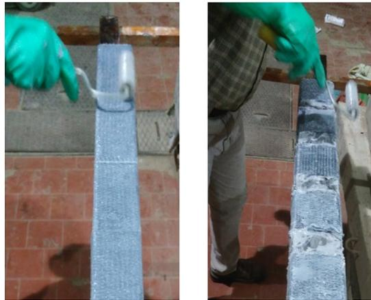
(a) Full strengthened specimen (b) Partial strengthened specimen
